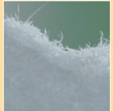
*Fibres sticking out from the edge of a sheet of paper*
